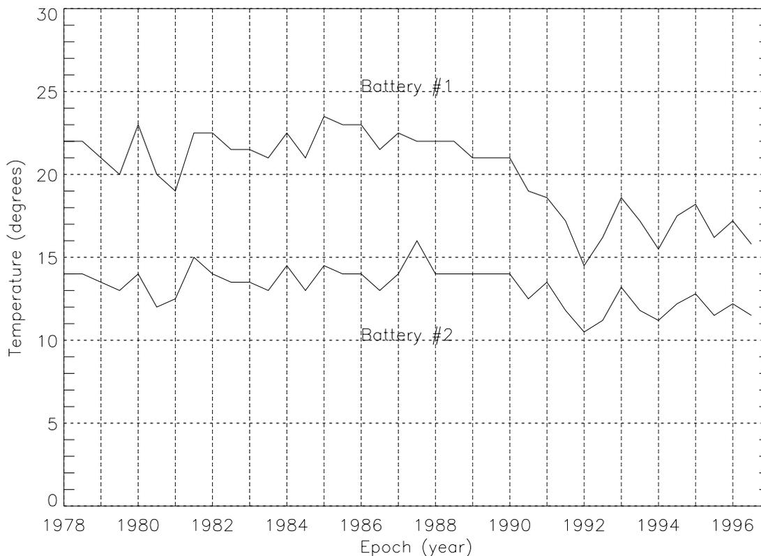
*Figure 5-8. History of average temperature of the batteries.*
