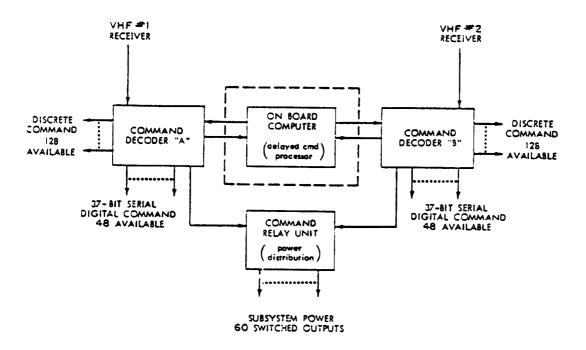
Figure 5-18. IUE Command Subsystem Block Diagram.
